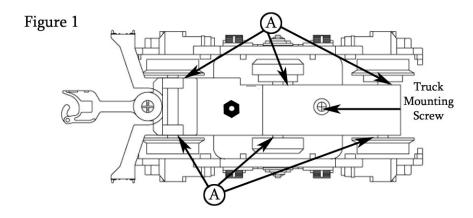
1. For the axles and coupler pivot points **Marked A**, we recommend that you lubricate with a small amount of light oil such as Bachmann E-Z Lube® #99984 Light Gear Oil. **Do not over-lubricate**.
